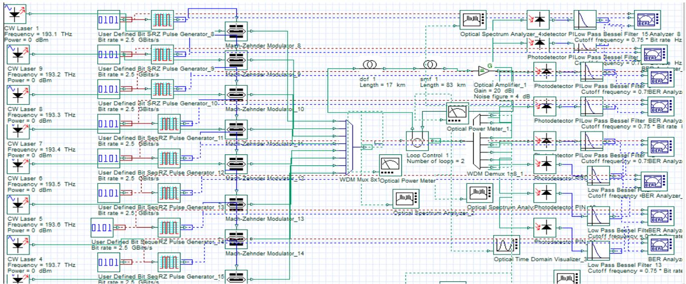
Figure 1: Simulation setup for 8-channel Dispersion Compensation Technique (DCF)
