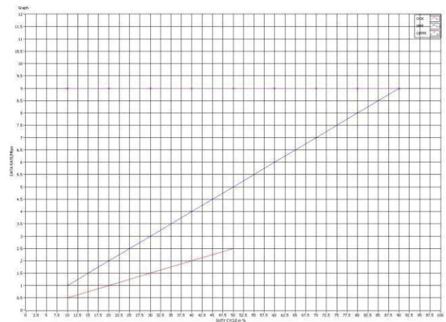
Figure 6. Lab View simulation of Data rate Vs Duty cycle for OOK & OPPM
