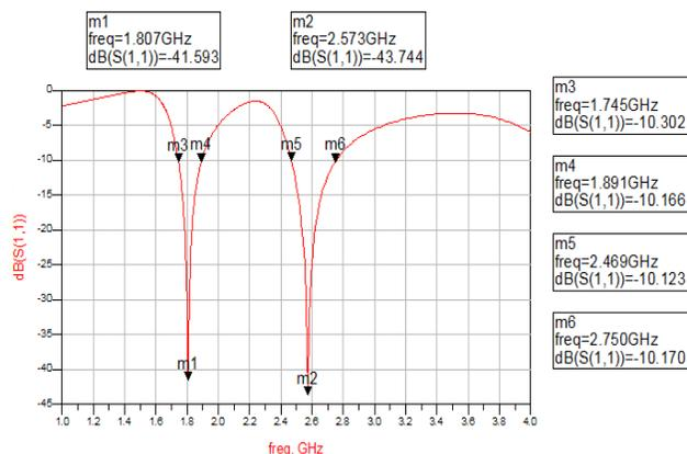
**Fig-3 simulation and measurement of return loss**
