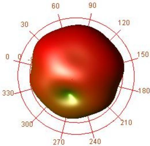
Fig 6. Measured radiation patterns for the proposed antenna at 2.573GHz
