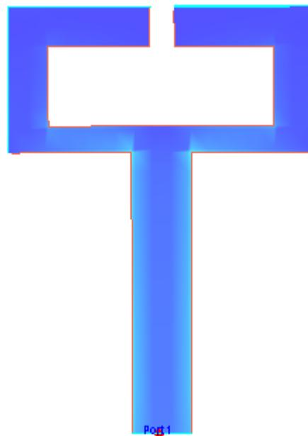
Fig 5. Measured current distribution for the proposed antenna at 1.807GHz
