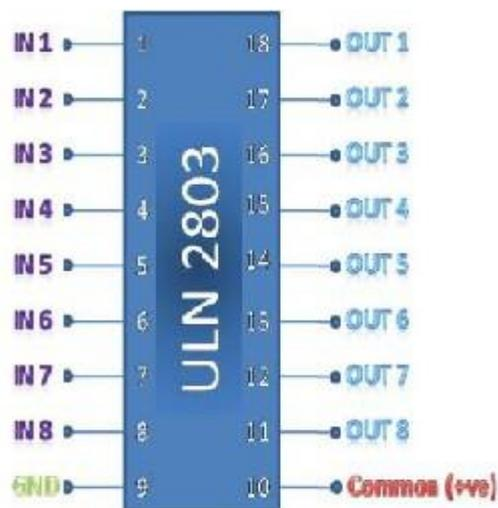
Fig. 2. ULN 2803 relay driver.
