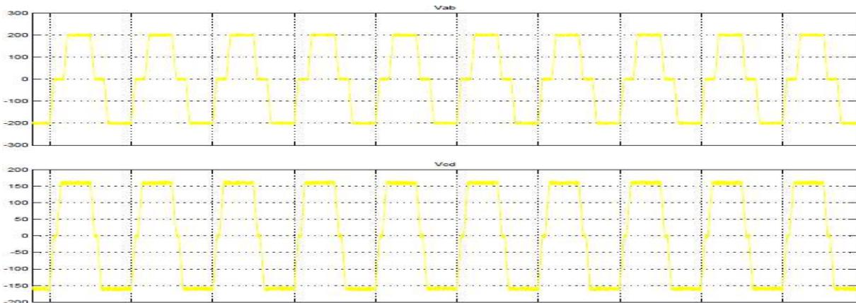
**Fig 6:** ZVS turn-ON of switches on the primary and secondary units
