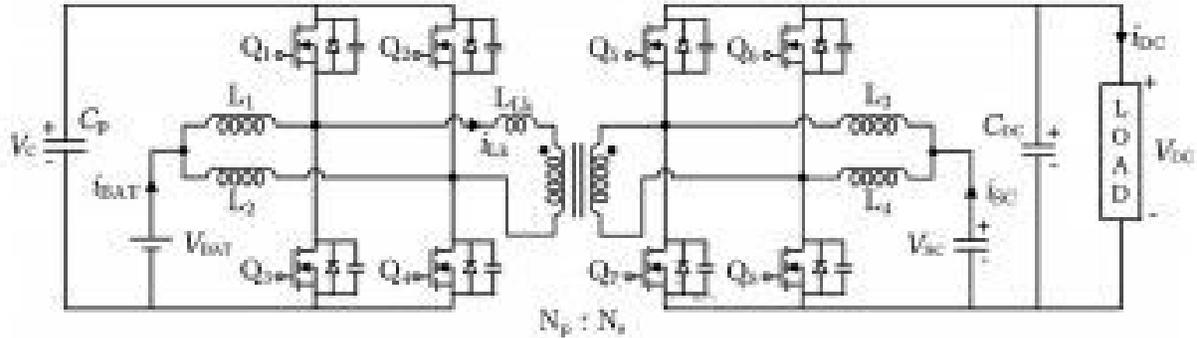
Fig 1: Topology of the multiport dc–dc converter proposed
