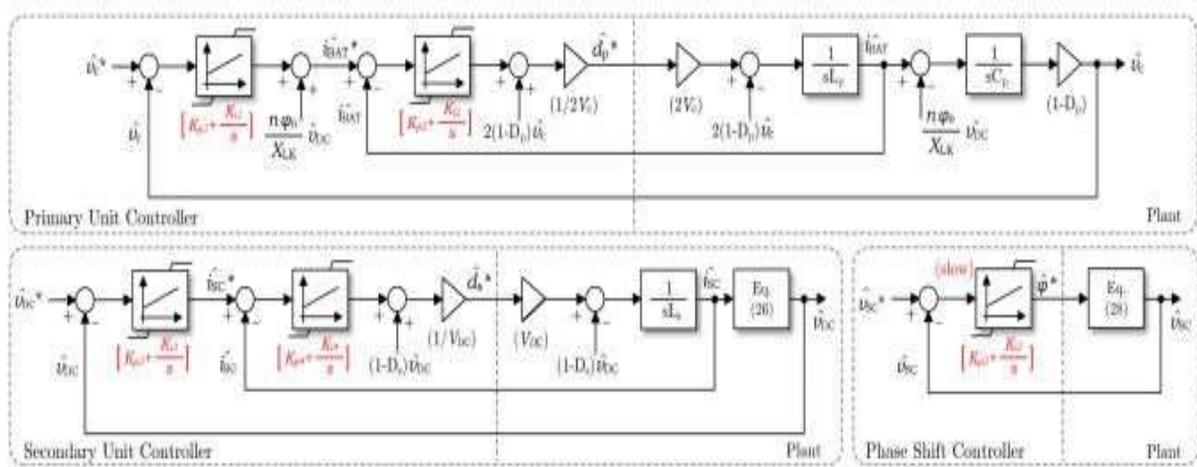
Fig 2: Detailed schematic of the control block diagram for the proposed high gain MPC
