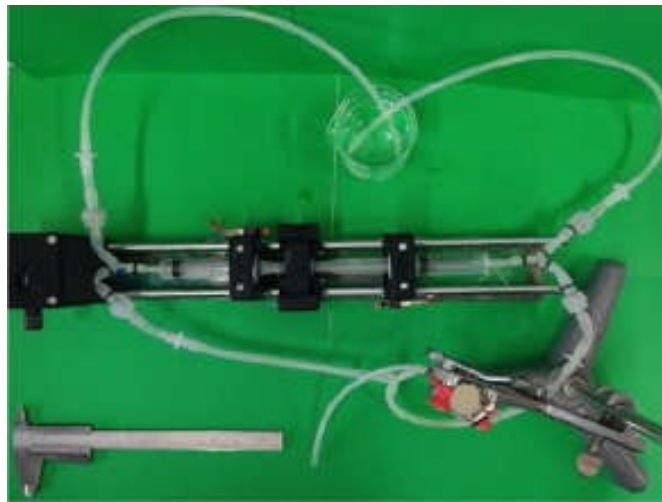
Figure 3.1 Pictorial Representation of PUSH-PULL SYRINGE PUMP [4] diagram
