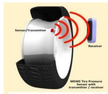
Fig 24: MEMMS tire pressure sensor
